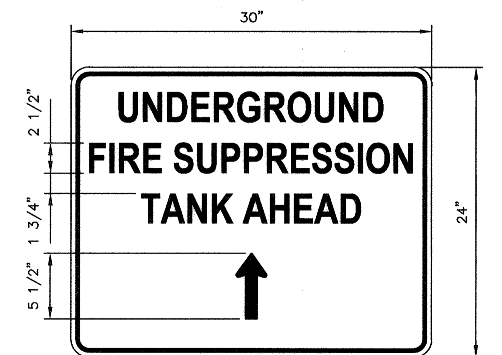
DETAIL: TYPICAL ADVANCE SIGNAGE SCALE: 1/2" = 1'-0"
