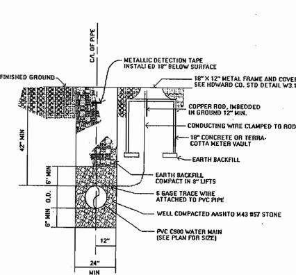
TRENCH FOR PVC PIPE AND CONTINUITY TEST STATION DETAIL
