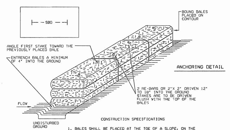
1. BALES SHALL BE PLACED AT THE TOE OF A SLOPE. ON THE CONTOUR, AND IN A ROW WITH THE ENOS OF EACH BALE TIGHTLY ABUTTING THE ADJACENT BALES.
