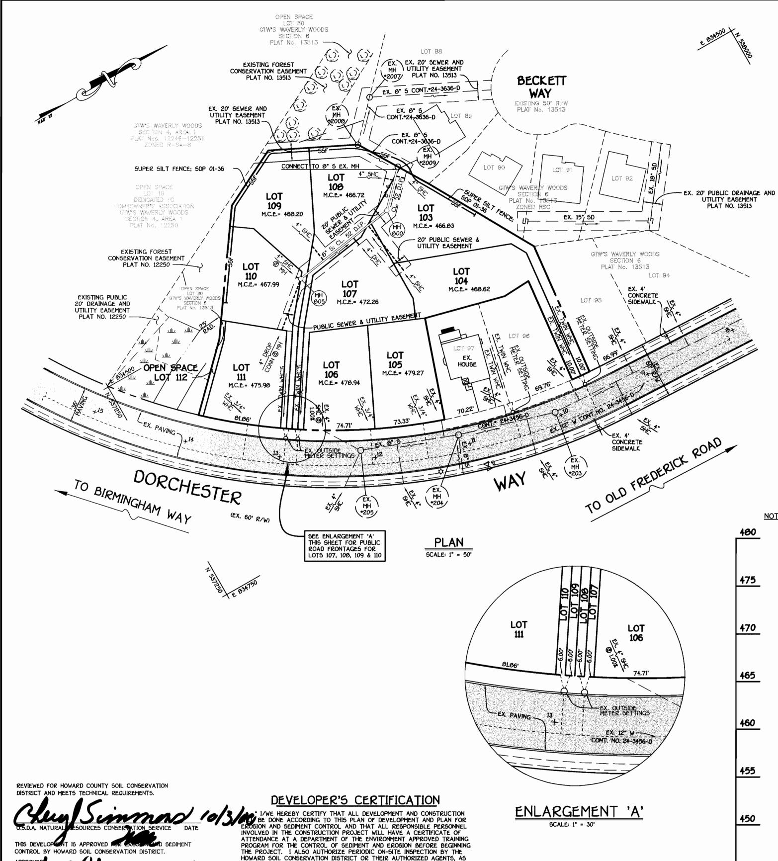
**QUANTITIES** A5-BUILT ESTIMATED QUANTITIES 8" SEWER (D.I.P.) 162.16 L.F. 4" SEWER 172 L.F. MANHOLES 2 EACH NAME OF UTILITY CONTRACTOR: SURVEY & DRAFTING DIVISION AS-BUILT DATE:
