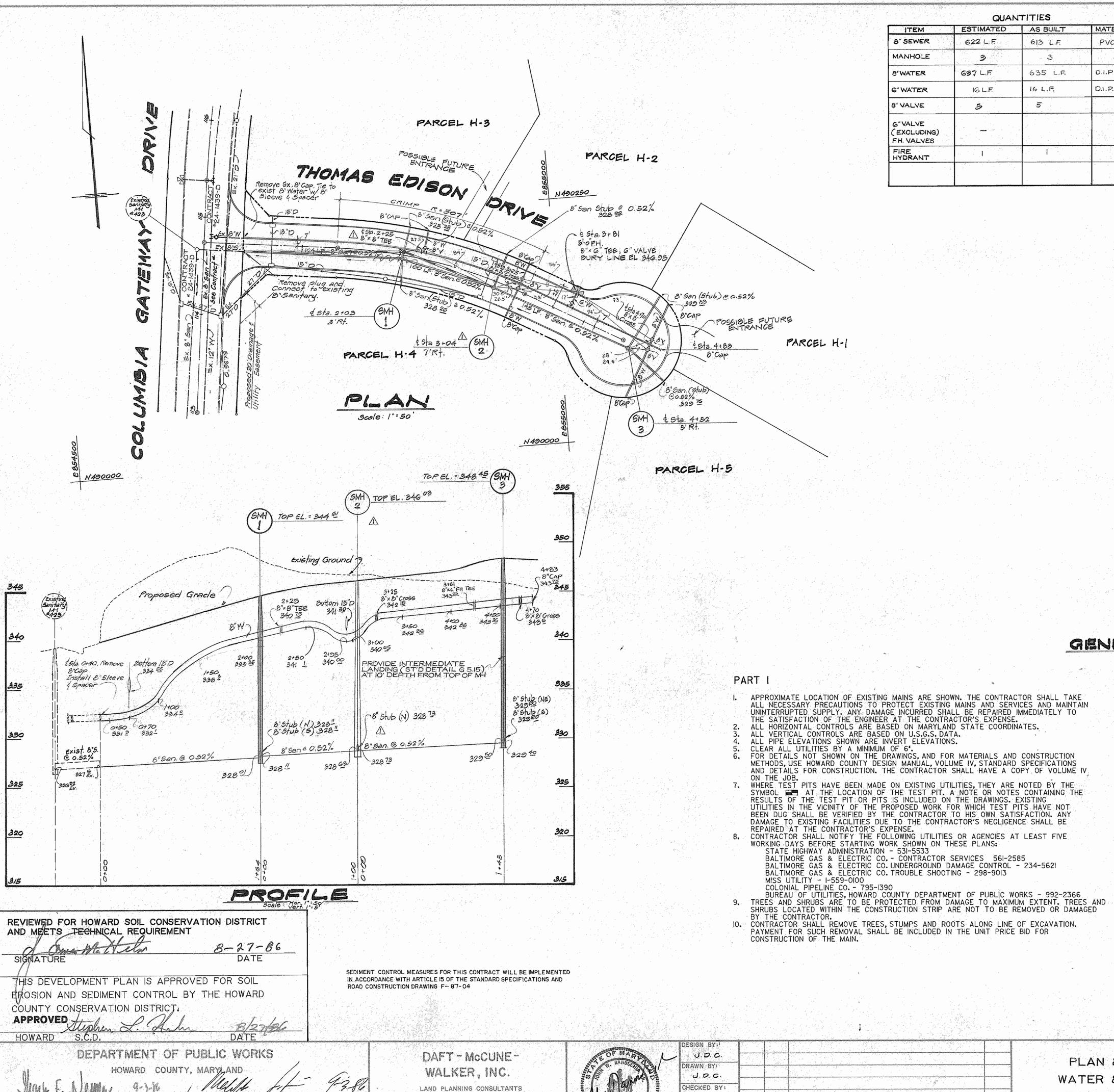
QUANTITIES ESTIMATED ITEM AS BUILT MATERIAL/SUPPLIER 8' SEWER 622 L.F. 613 L.F. ATLANTIC MANHOLE - 3 3 637 L.F. 635 L.F. GRIFFIN 8"WATER GRIFFIN 16 L.F. G' WATER 16 L.F MI & H VALVE 8" VALVE 6"VALVE (EXCLUDING) FH. VALVES FIRE HYDRANT M&H VALVE
