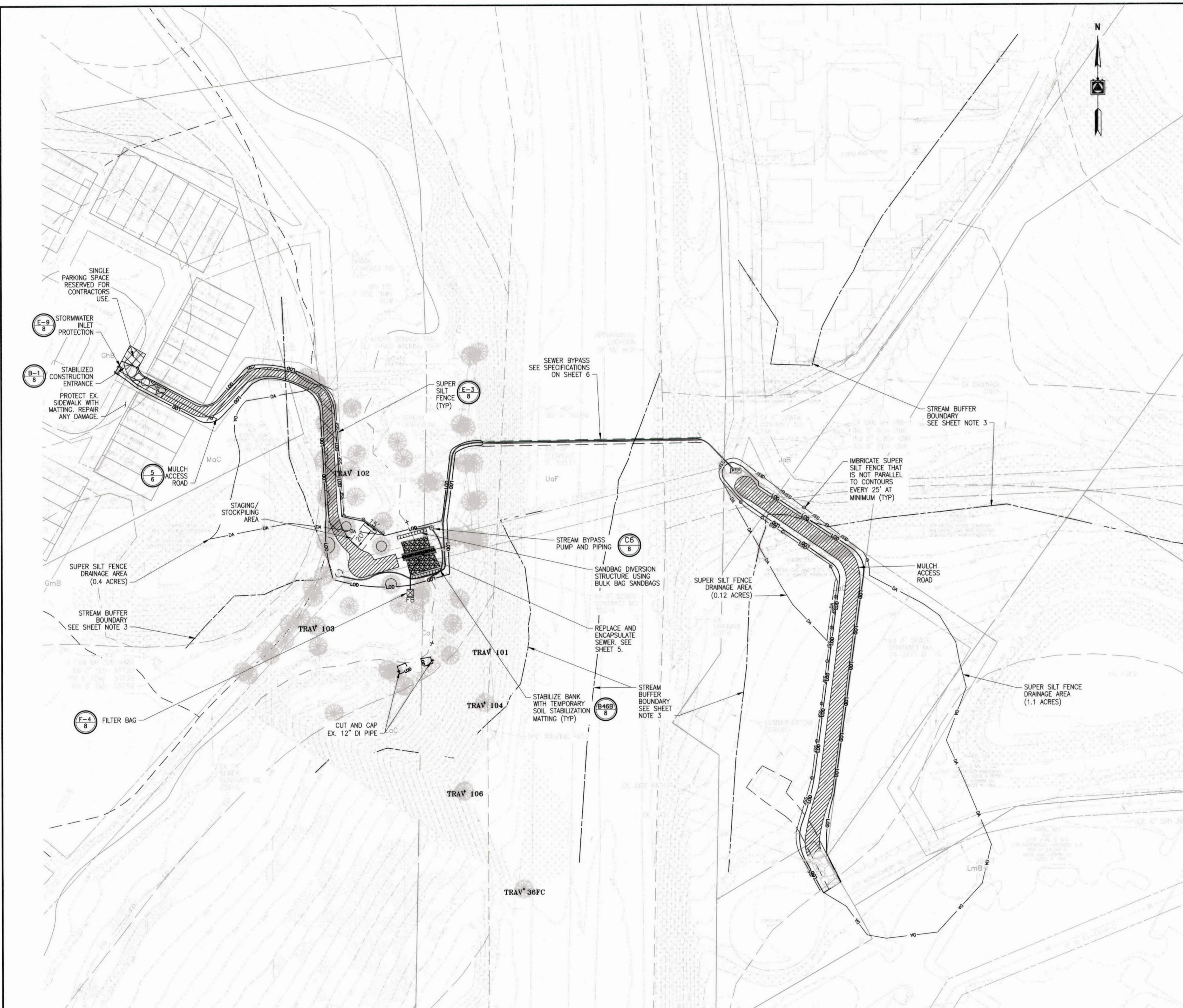
EROSION AND SEDIMENT CONTROL PLAN SCALE: 1"=50'
