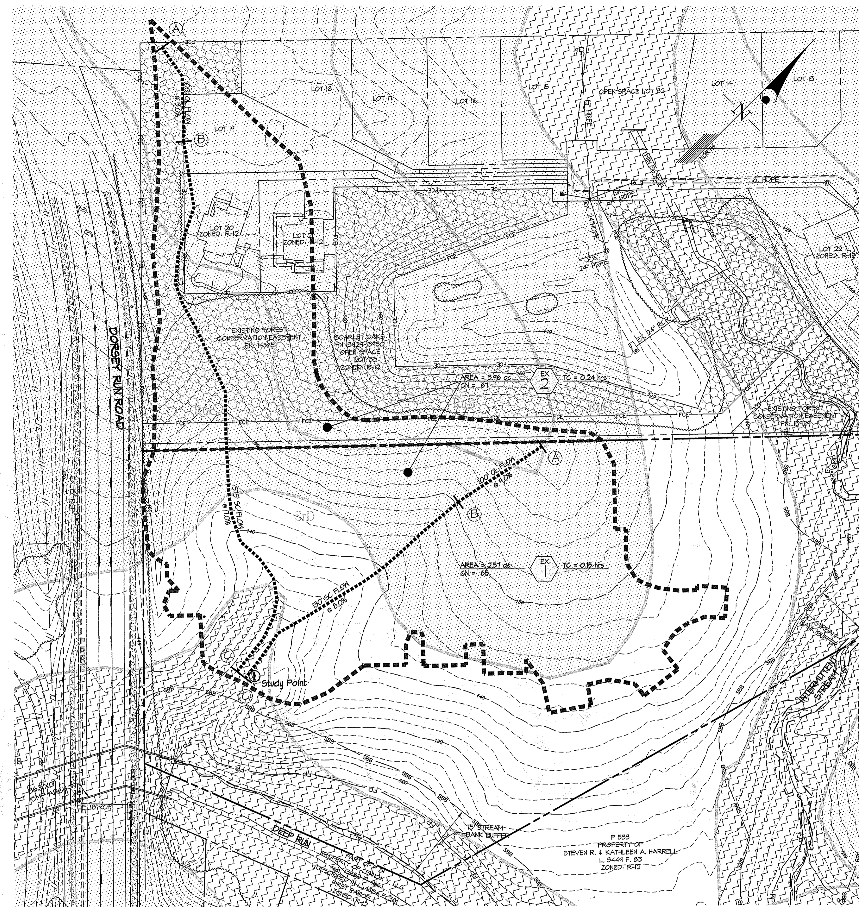
EXISTING CONDITIONS DRAINAGE AREA MAP
