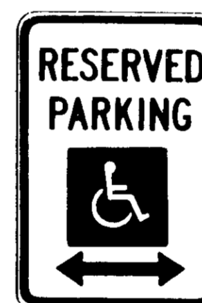
HANDICAPPED PARKING SIGN DETAIL SCALE: 1/2" = 1'-0"
