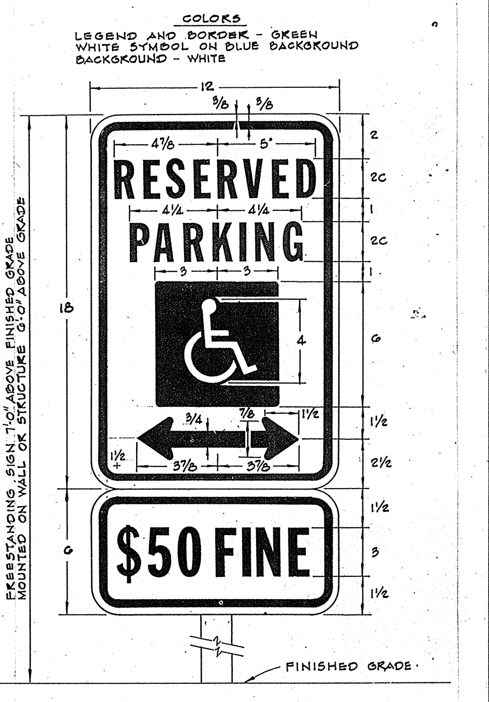
HANDICAPPED PARKING SIGN NO SCALE
