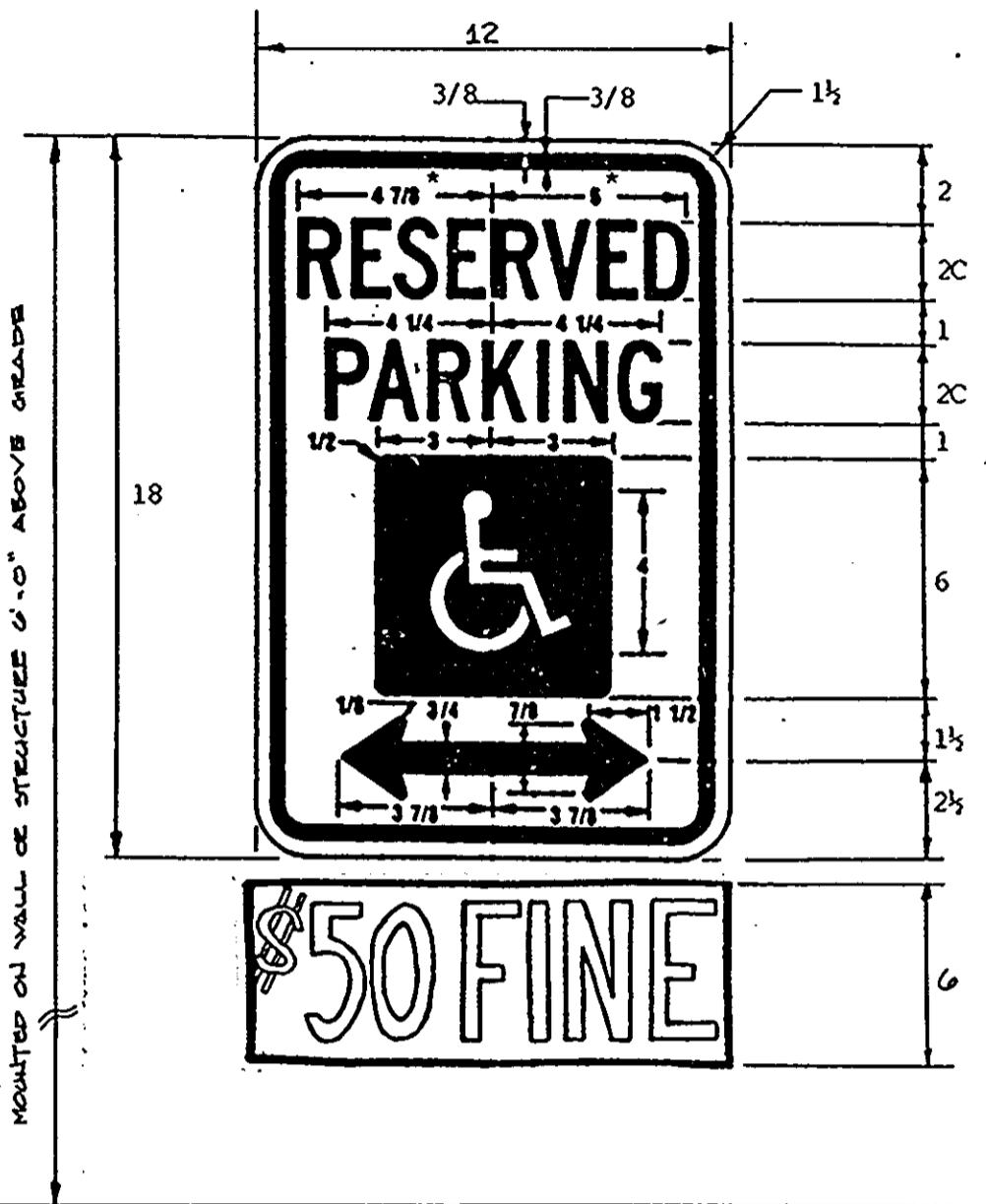
COLORS: LEGEND AND BORDER - GREEN WHITE SYMBOL ON BLUE BACKGROUND BACKGROUND - WHITE * - REDUCE SPACING 50 PERCENT
