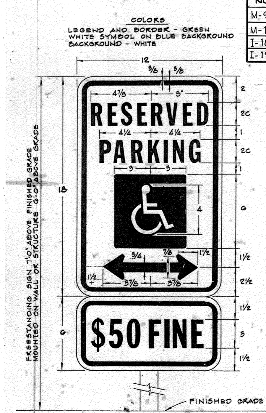
HANDICAPPED PARKING SIGN NO SCALE
