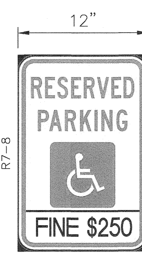
ACCESSIBLE SIGN MOUNTED ON U-CHANNEL SIGN POST AT END OF ACCESSIBLE SPACE BOTTOM OF SIGN MUST BE 6" MIN. ABOVE GROUND (NOT TO SCALE)
