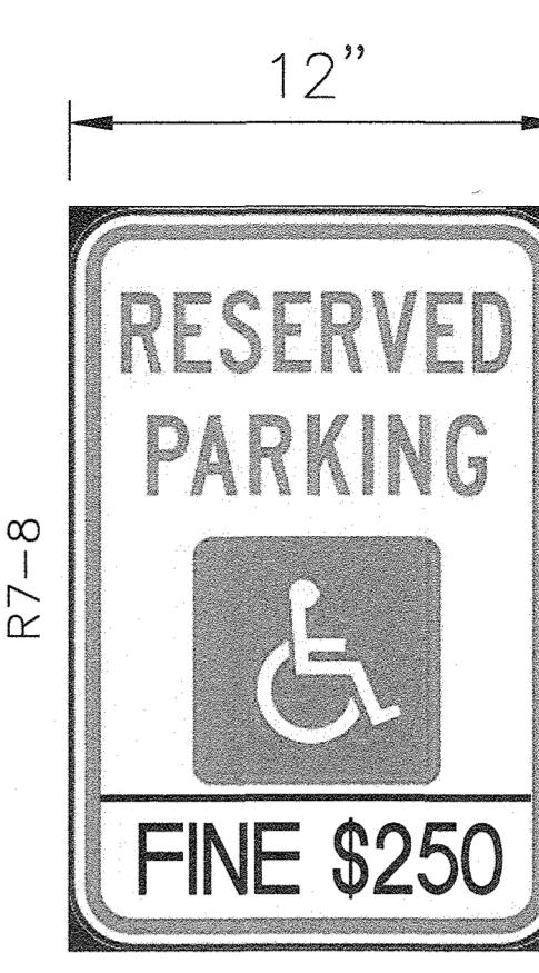
VAN ACCESSIBLE SIGN MOUNTED ON U-CHANNEL SIGN POST AT END OF ACCESSIBLE SPACE BOTTOM OF SIGN MUST BE 6" MIN. ABOVE GROUND (NOT TO SCALE)
