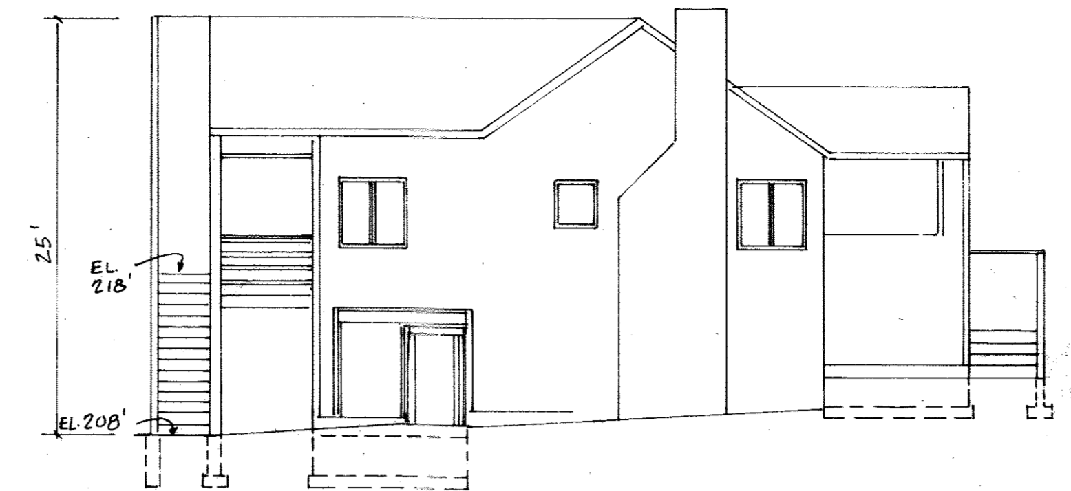
EAST ELEVATION: SCALE: 1/8"=1'-0" TWO STORY OFFICE ADDITION
