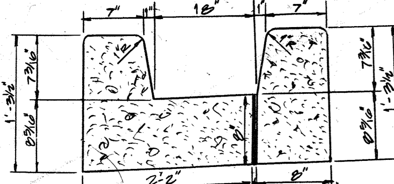
CURB OPENING DETAIL NOT TO SCALE
