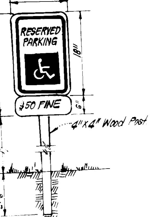
HANDICAP PARKING SIGN DETAIL NO SCALE
