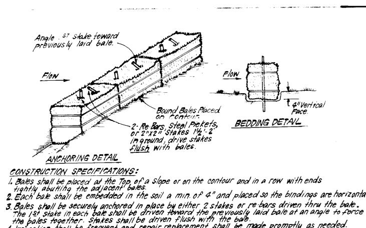
1. Bales shall be placed at the Top, of a Slope or on the contour and in a row with ends
