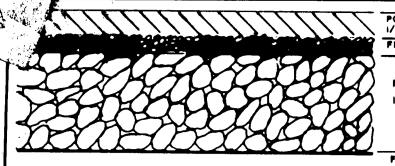
POROUS ASPHALT COURSE 1/2" TO 3/4" ASSRESATE ASPHALTIC MIX FILTER COURSE 1/2" AGGREGATE " TO 2" AGGREGATE
