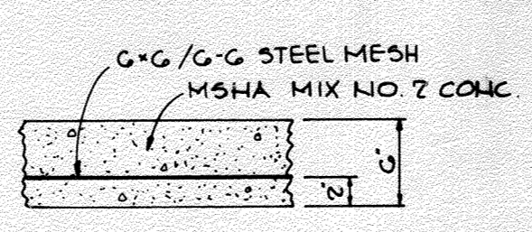
DUMPSTER PAD DETAIL NO SCALE
