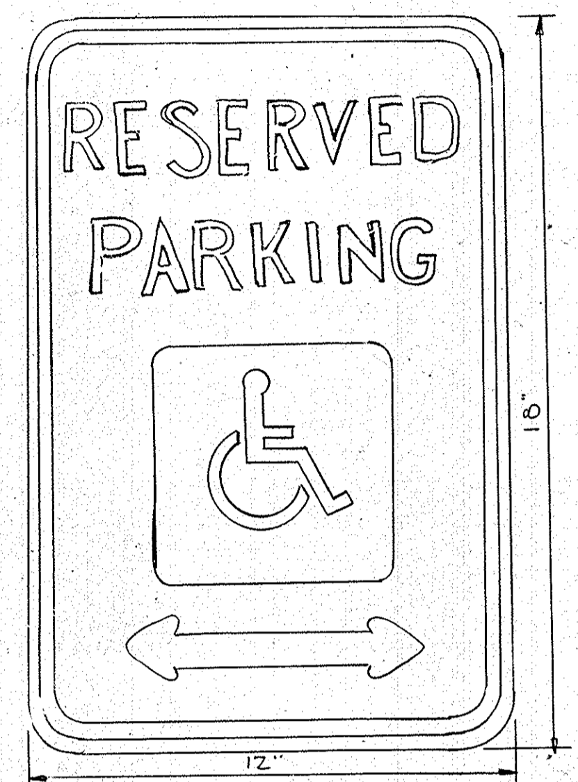
HANDICAPPED PARKING SIGN DETAIL SHOWN THUS ON PLAN *
