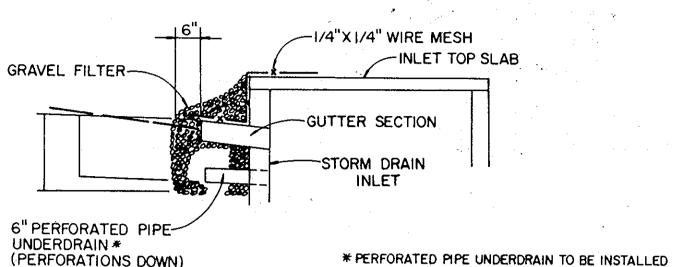
STONE FILTER INLET PROTECTION DETAIL
