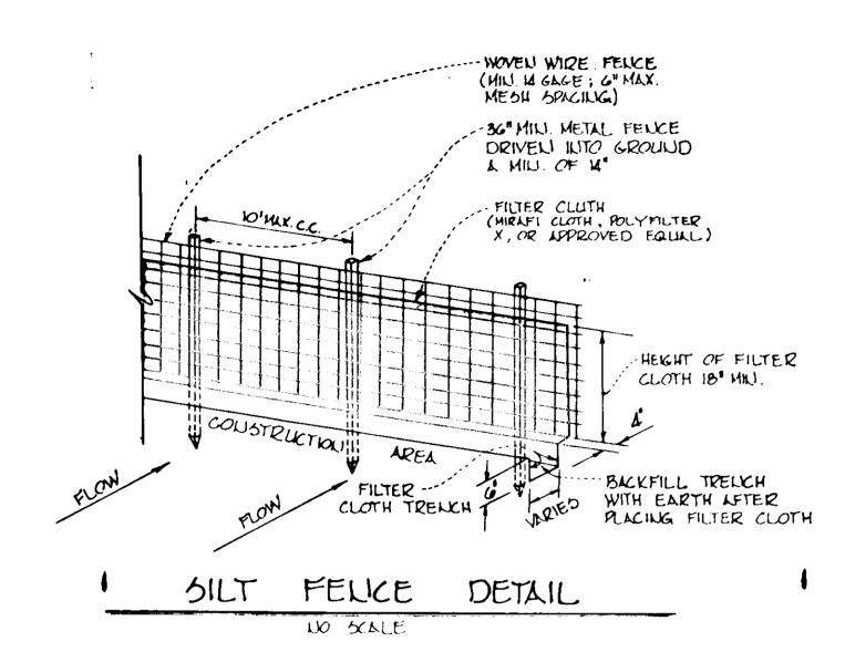
I WOVEN WIRE FELICE TO BE FASTENED SECURELY TO FENCE POSTS BY USE OF WIRE TIES. 7. FILTER CLOTH TO BE FASTELIED SECURELY TO WOVEN WIRE FELICE BY USE OF WIRE TIES.
