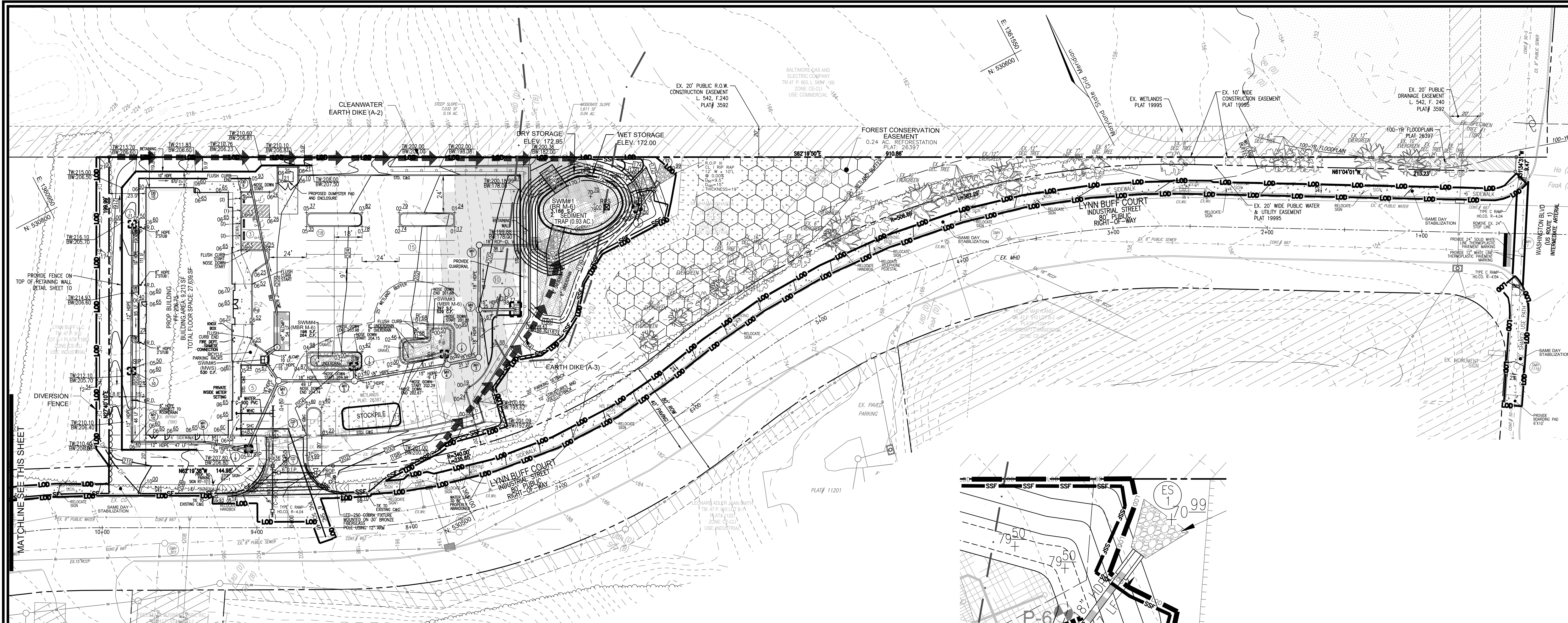
EROSION AND SEDIMENT CONTROL PLAN
