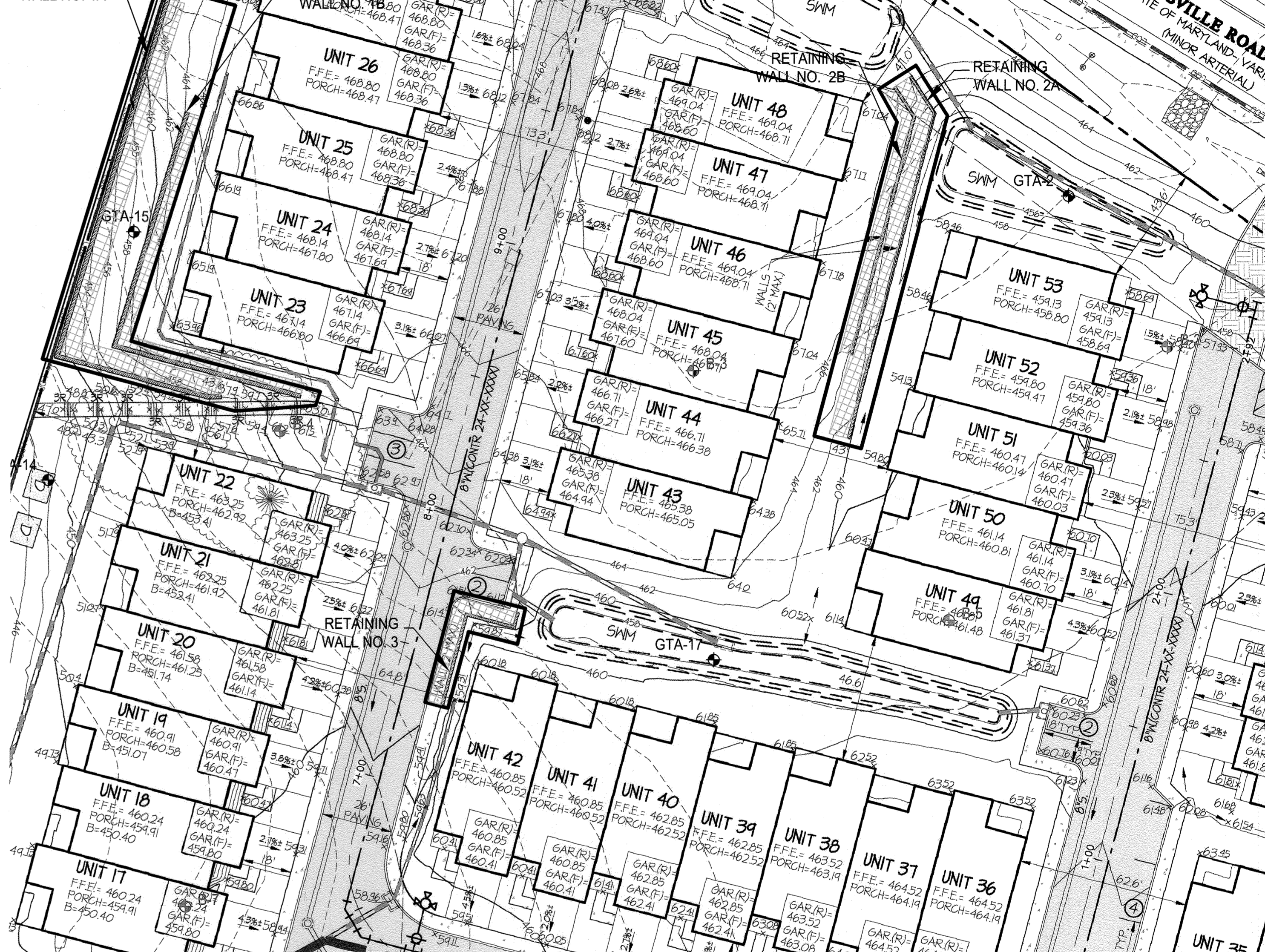
RETAINING WALL LOCATION PLAN
