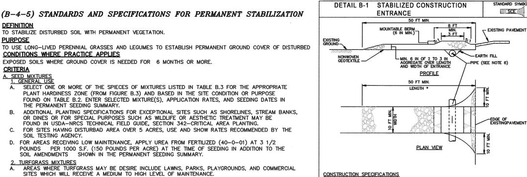
PLACE STABILIZED CONSTRUCTION ENTRANCE IN ACCORDANCE WITH THE APPROVED PLAN. VEHICLES MUST TRAVEL OVER THE ENTIRE LENGTH OF THE SCE. USE MINIMUM LENGTH OF 50 FEET (\*30 FEET FOR SINGLE RESIDENCE LOT). USE MINIMUM WIDTH OF 10 FEET. FLARE SCE 10 FEET MINIMUM AT THE EXISTING ROAD TO PROVIDE A TURNING RADIUS.
