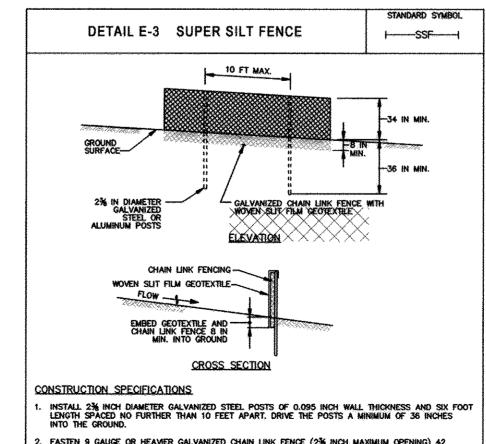
FASTEN 9 GAUGE OR HEAVER GALVANIZED CHAIN LINK FENCE (2% INCH MAXIMUM OPENING) 42 INCHES IN HEIGHT SECURELY TO THE FENCE POSTS WITH WIRE TIES OR HUG RINGS.
