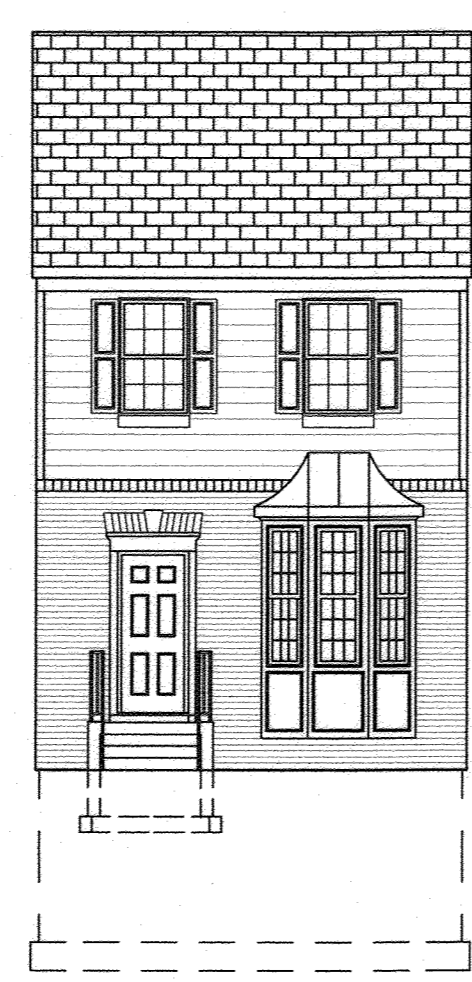
FRONT ELEVATION (BRICK WATER TABLE (1)) NO SCALE
