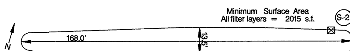
SWM-2 Micro-Bioretenion Dimensions NOT TO SCALE
