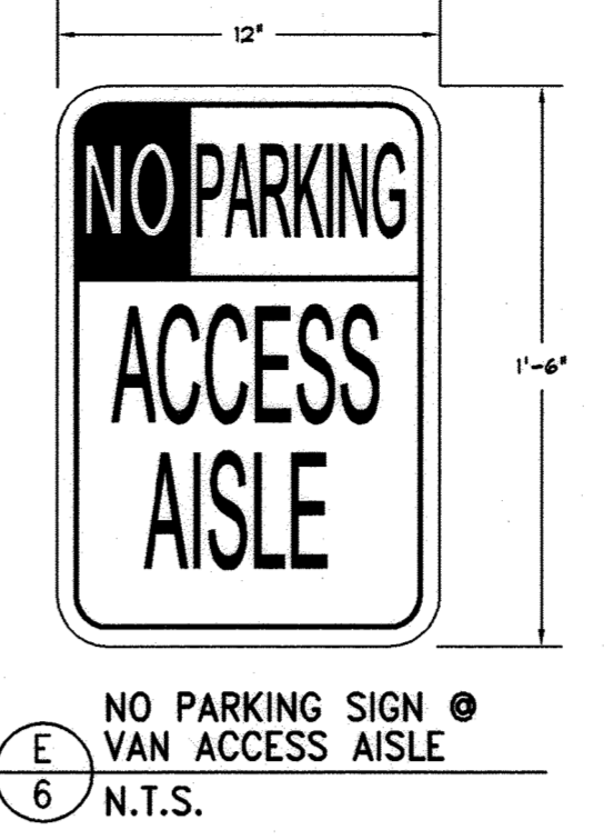
E NO PARKING SIGN @ VAN ACCESS AISLE 6 N.T.S.
