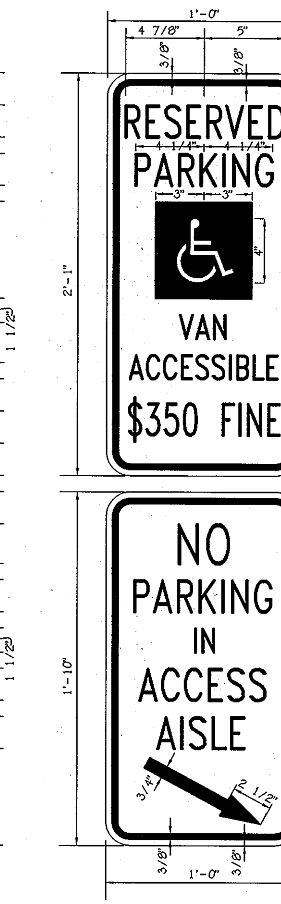
10 VAN ACCESSIBLE PARKING SIGN DETAIL NO SCALE
