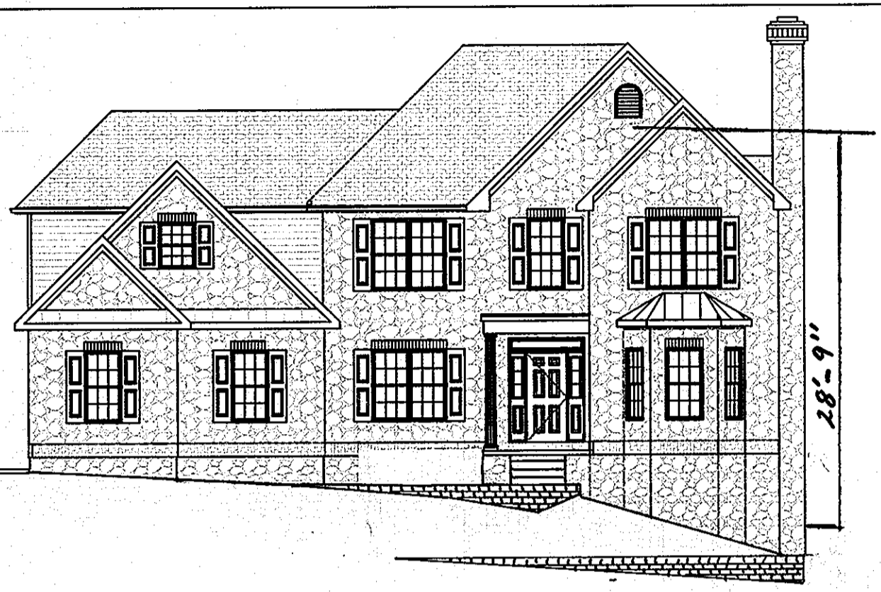
BUILDING ELEVATION SCALE: 1" = 10'
