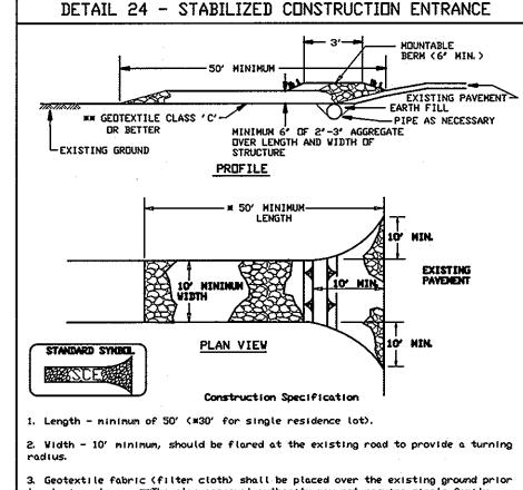
to placing stone. \*\*The plan approval authority may not require single family . Stone - crushed aggregate (2' to 3') or reclaimed or recycled concrete
