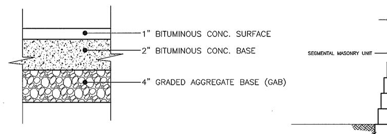
COMMON DRIVEWAY PAVING DETAIL NOT TO SCALE
