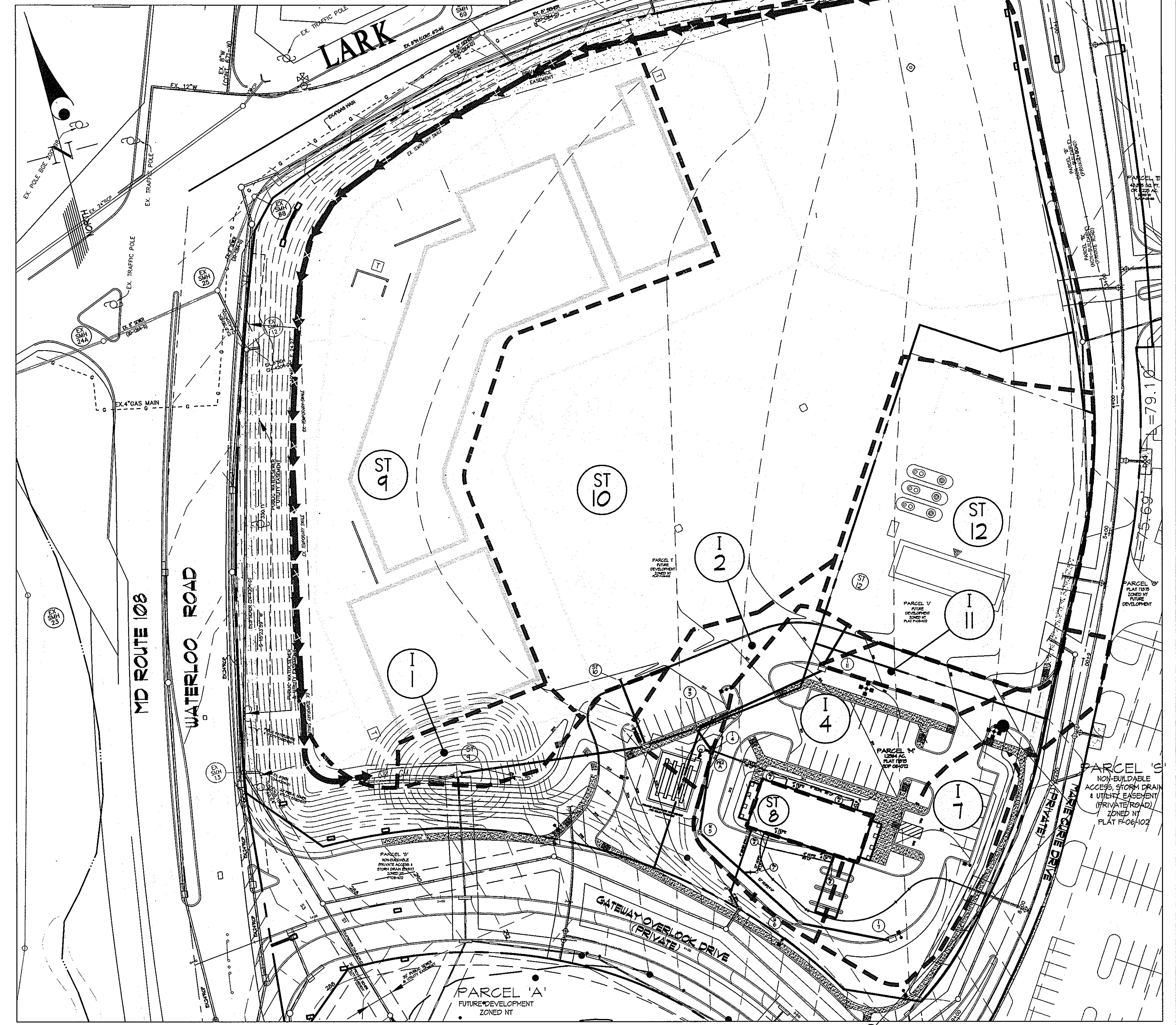
STORM DRAIN DRAINAGE AREA MAP SCALE: 1" = 50'
