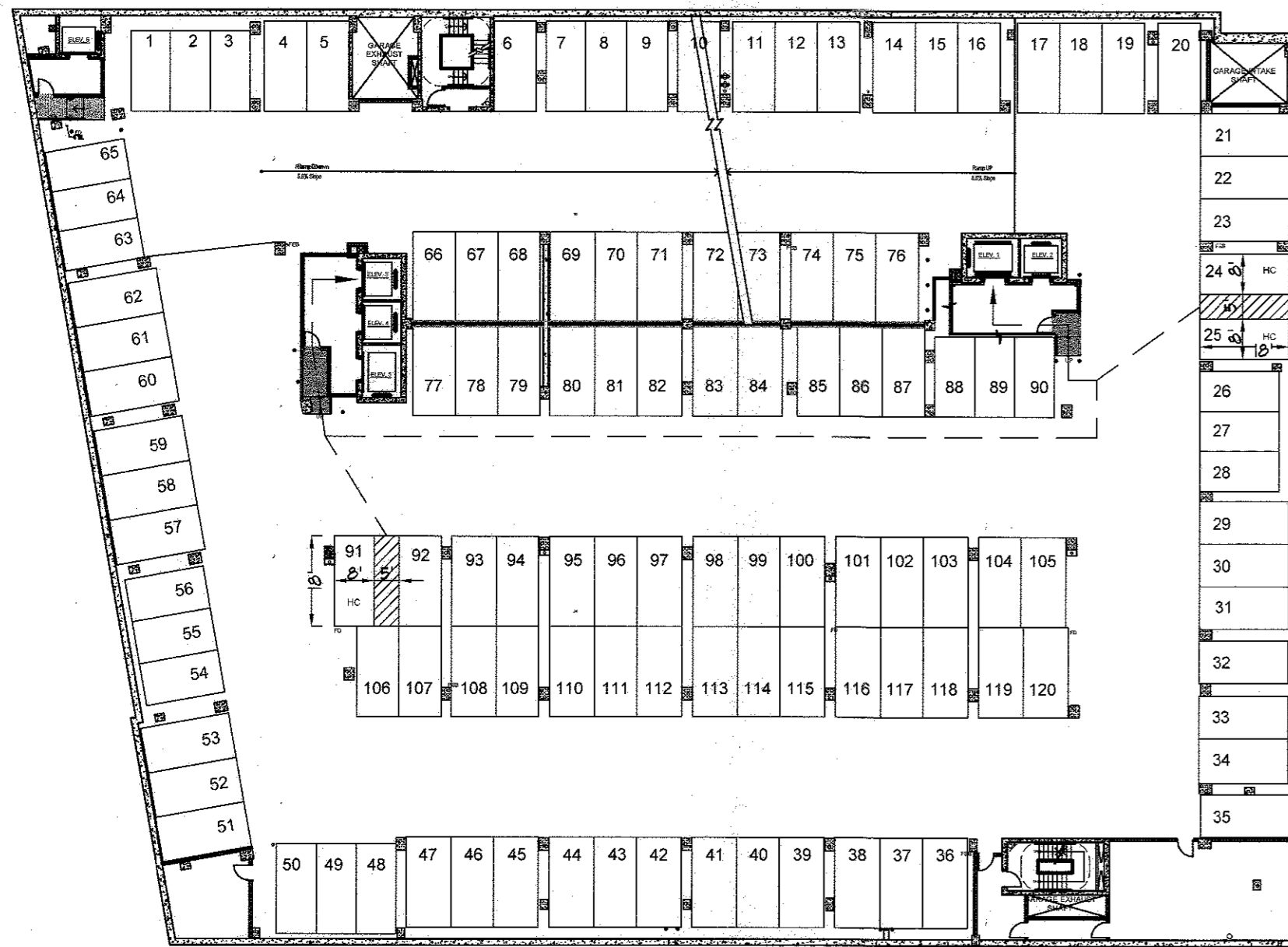
▲ PARKING LEVEL 1 - 117 SPACES + 3 HANDICAP SPACES = 120 SPACES SCALE: 1" = 30'
