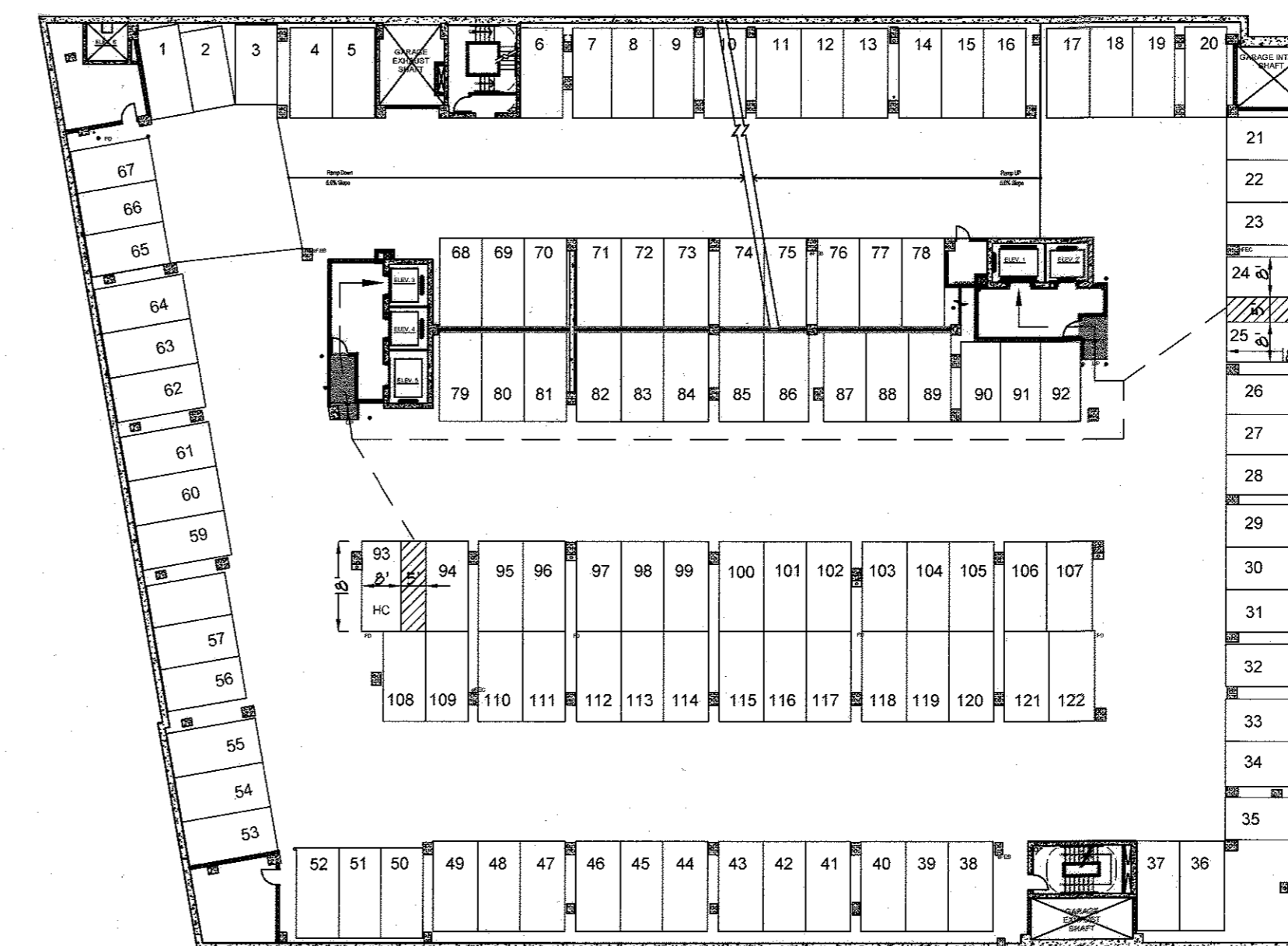
▲ PARKING LEVEL 3 - 119 SPACES + 3 HANDICAP SPACES = 122 SPACES SCALE: 1" = 30'
