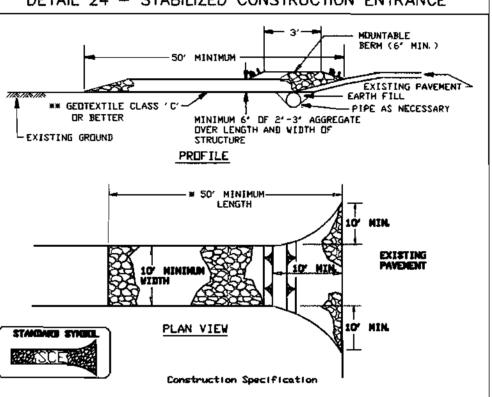
). Geotextile fabric (filter cloth) shall be placed over the existing ground prior to placing stone. \*\*The plan approval authority may not require single family residences to use geotextile.
