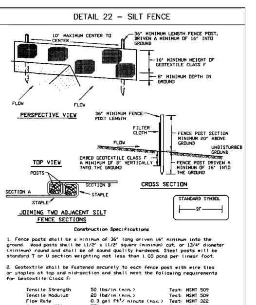
3. Where ends of geotextile fabric come together, they shall be overlapped, folded and stapled to prevent sediment bypass. 4. Silt Fence shall be inspected after each rainfall event and maintained when bulges occur or when sediment accumulation reached 50% of the fabric height.
