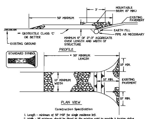
2. Width - 10' minimum, should be flared at the existing road to provide a turning radius. 3. Geotextile fabric (filter cloth) shall be placed over the existing ground prior to placing stone. \*\*The plan approval authority may not require single family
