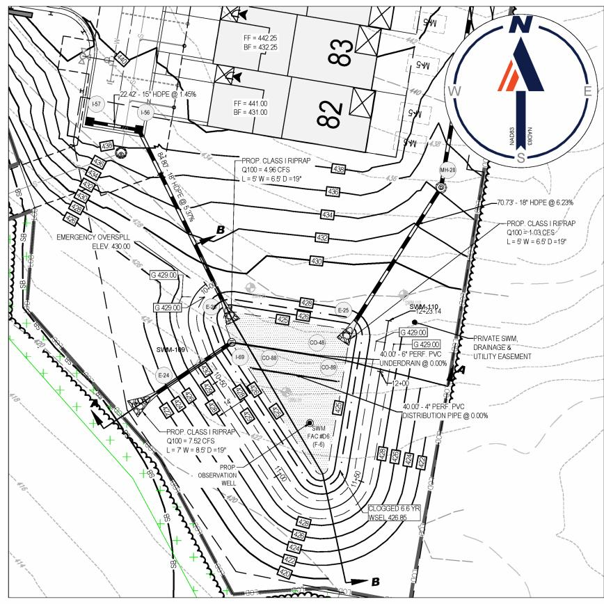
PLAN VIEW - SWM FACILITY #D6 - SURFACE SAND FILTER (F-1)
