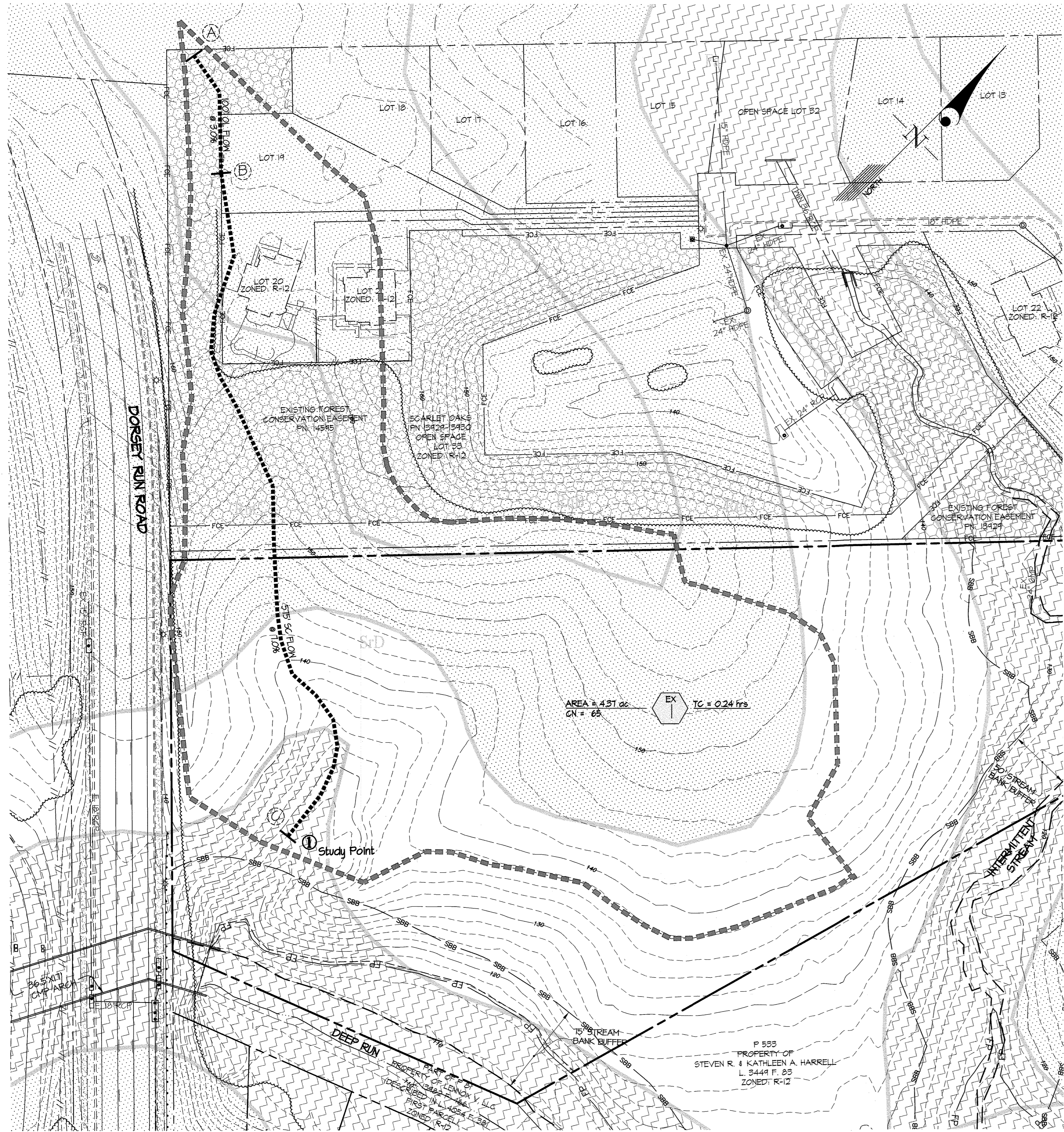
EXISTING CONDITIONS DRAINAGE AREA MAP
