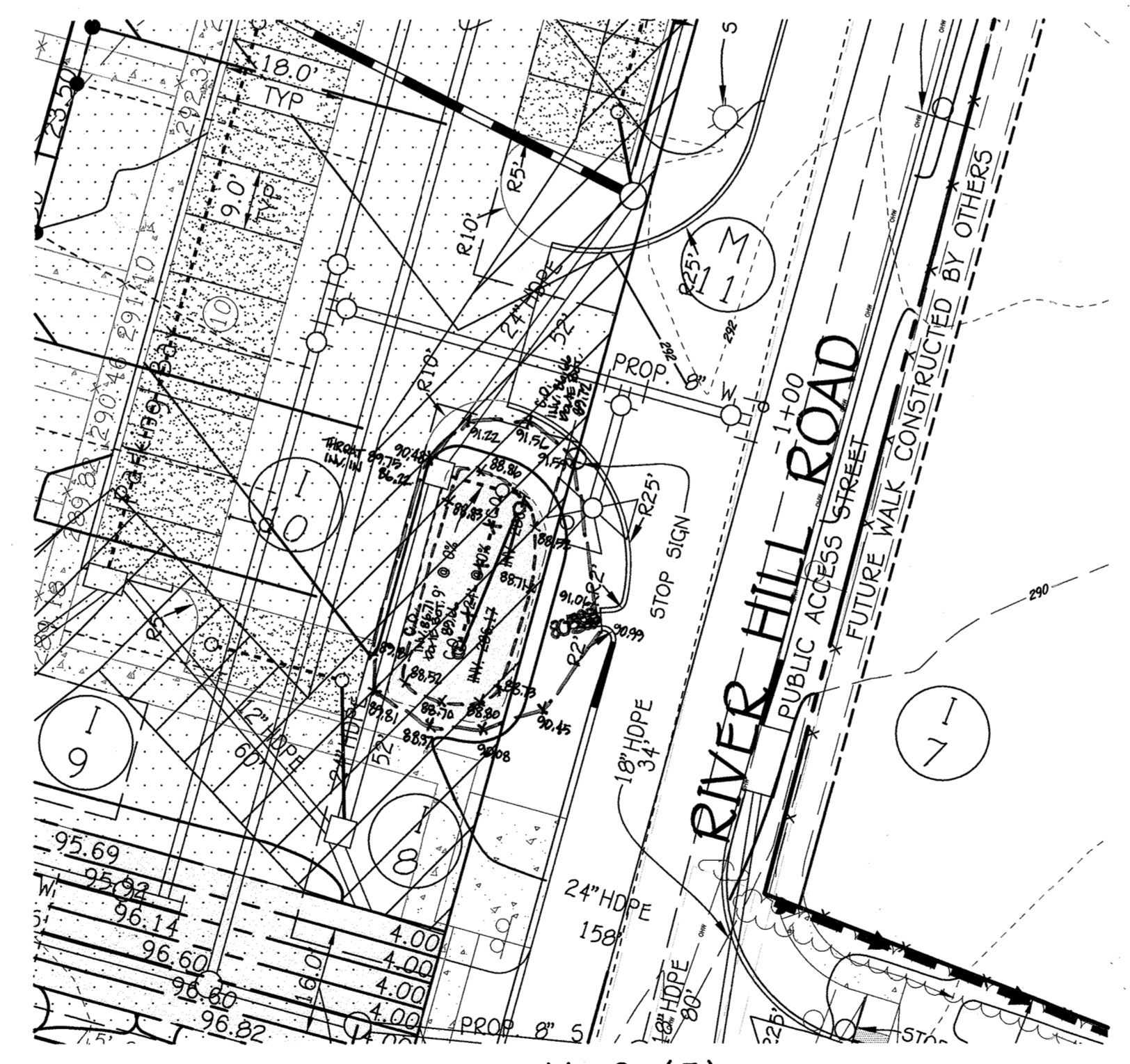
M-6 (5) (MICRO BIO-RETENTION FACILITY) SCALE: 1" = 20' DRAINAGE AREA: 6,879 SqFt. FILTER AREA: 606 SqFt. ELEVATION: 289 PERIMETER: 99' WEIR ELEVATION: 290
