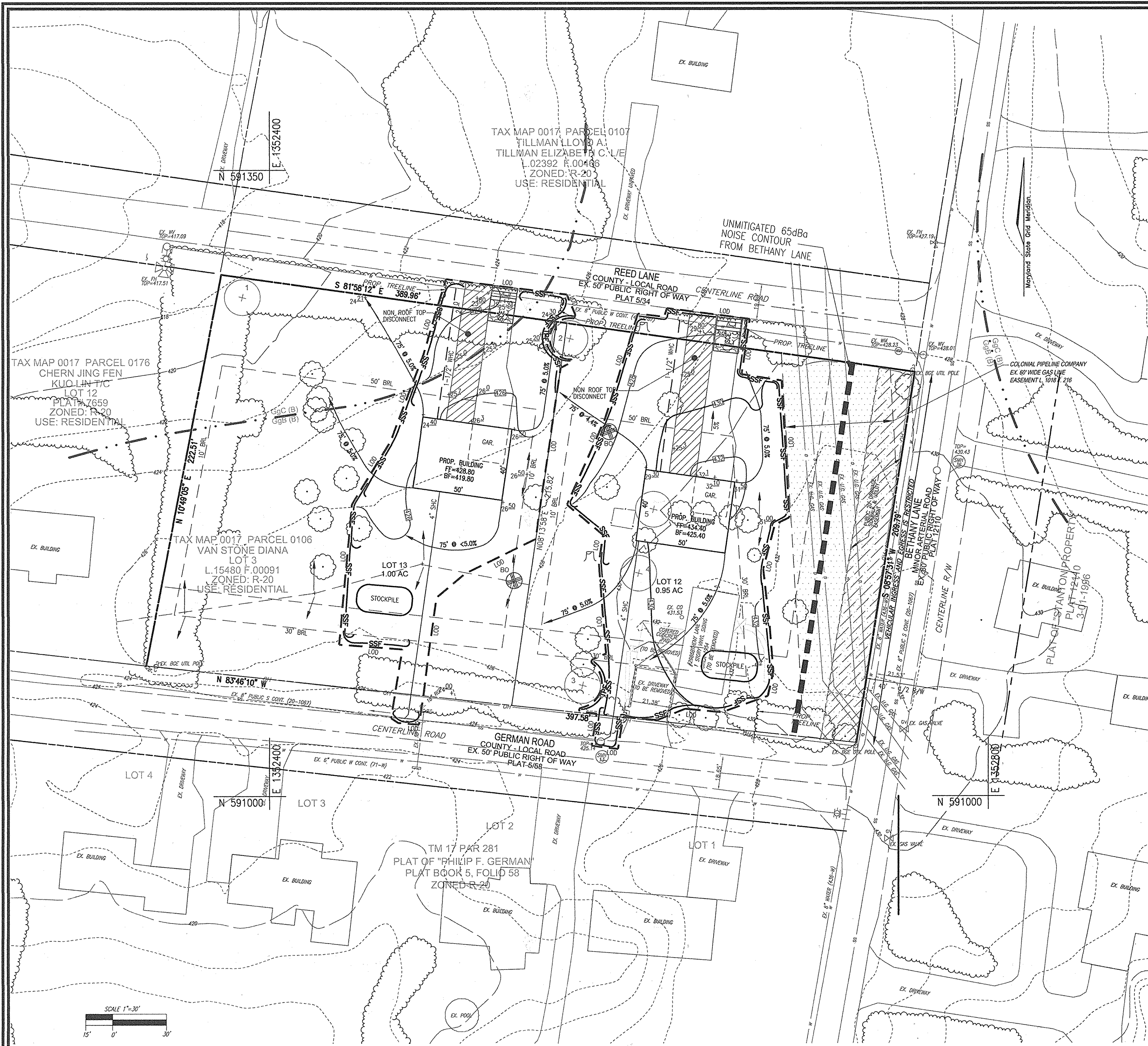
GRADING, SOILS MAP, SWM PLAN SCALE: 1" = 30'
