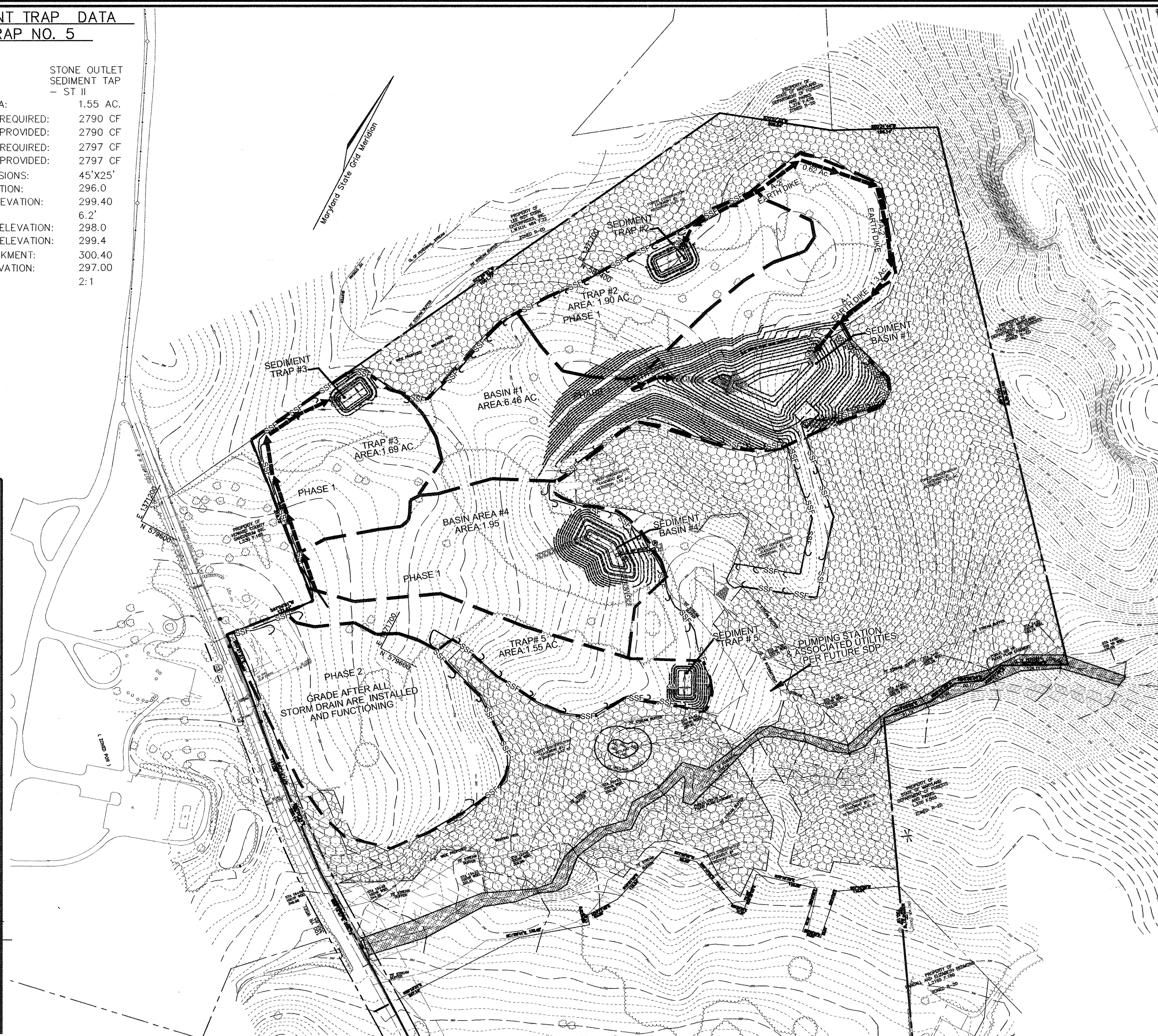
PRE-CONSTRUCTION TEMPORARY SWM DRAINAGE AREA MAP SCALE: 1"=100'
