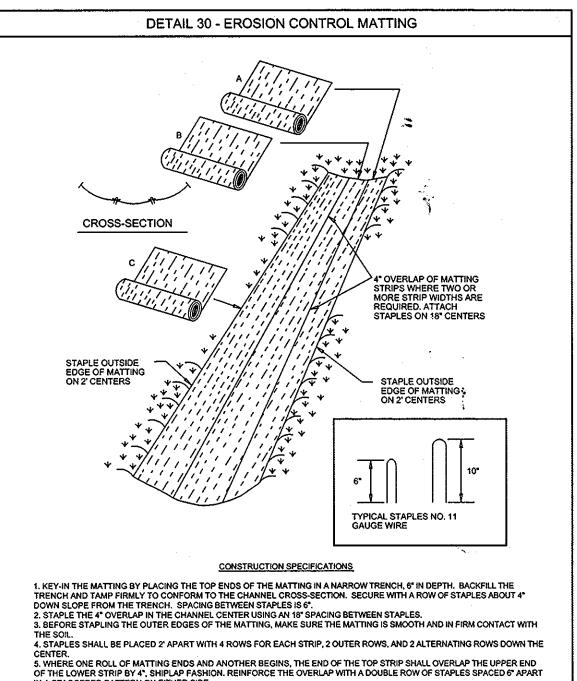
IN A STAGGERED PATTERN ON EITHER SIDE. 6. THE DISCHARGE END OF THE MATTING LINER SHOULD BE SIMILARLY SECURED WITH 2 DOUBLE ROWS OF STAPLES.
