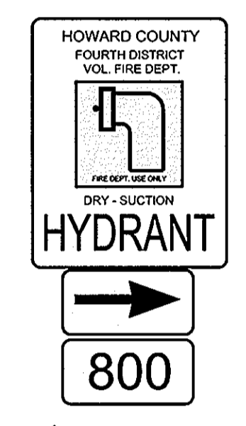
DRY HYDRANT SIGN
