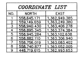
NOTE: COORDINATES AND GRID TICS SHOWN HEREON ARE BASED ON NAD '83 AND ARE IN FEET, TO CONVERT TO METERS DIVIDE BY 3.28083333.
