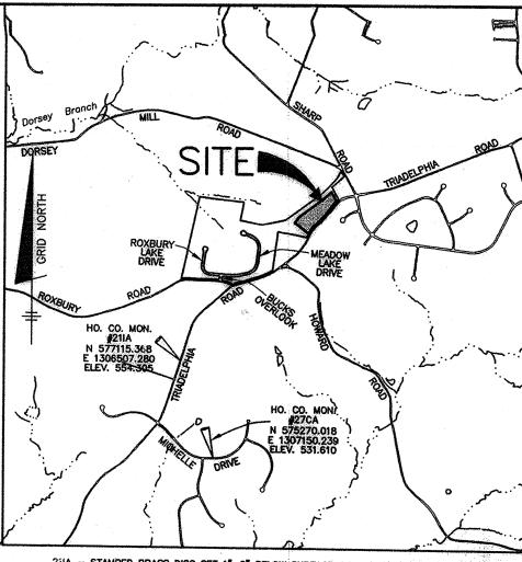
STAMPED BRASS DISC SET 1"-2" BELOW SURFACE ON A CONCRETE COLUMN (3' DEEP) LOCATED 4' FROM WEST EDGE OF TRIADELPHIA ROAD 99' FROM BGE POLE \$134679. 27CA - STAMPED BRASS DISC SET 1"-2" BELOW SURFACE ON A CONCRETE COLUMN (3' DEEP)
