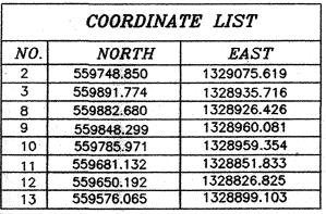
NOTE: COORDINATES AND GRID TICKS SHOWN HEREON ARE BASED ON NAD'83 AND ARE IN FEET.
