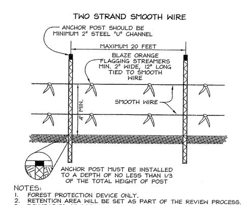
BOUNDARIES OF RETENTION AREA SHOULD BE STAKED AND FLAGGED PRIOR TO INSTALLING DEVICE.
