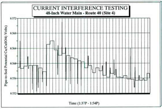
Figure 13. Detailed Current Interference Test Results for Site 4 from 1:20PM - 1:54PM
