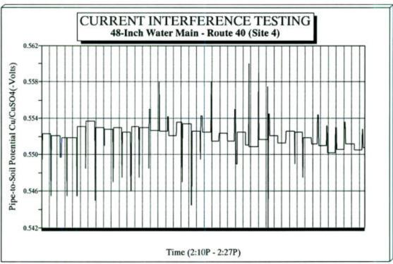
Figure 14. Detailed Current Interference Test Results for Site 4 from 1:54PM - 2:27PM
