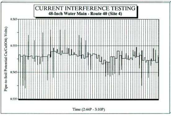
Figure 15. Detailed Current Interference Test Results for Site 4 from 2:27PM - 3:10PM
