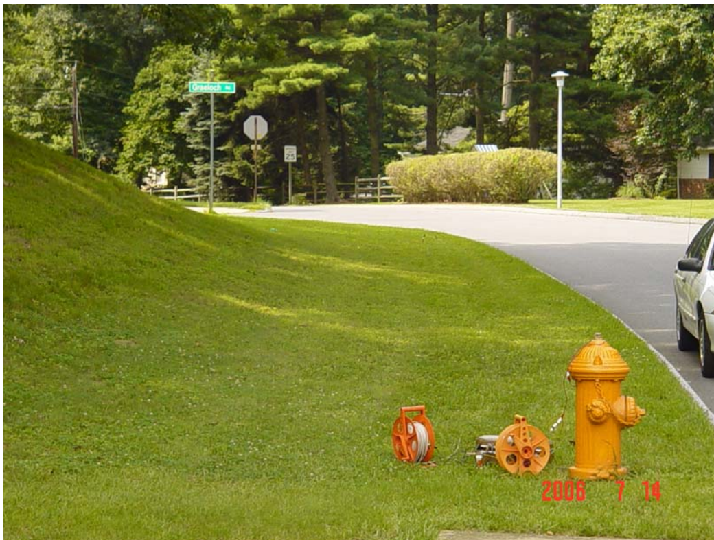
Figure 76 - Measuring stray currents near the Helmart Drive/Grae Loch Road intersection
