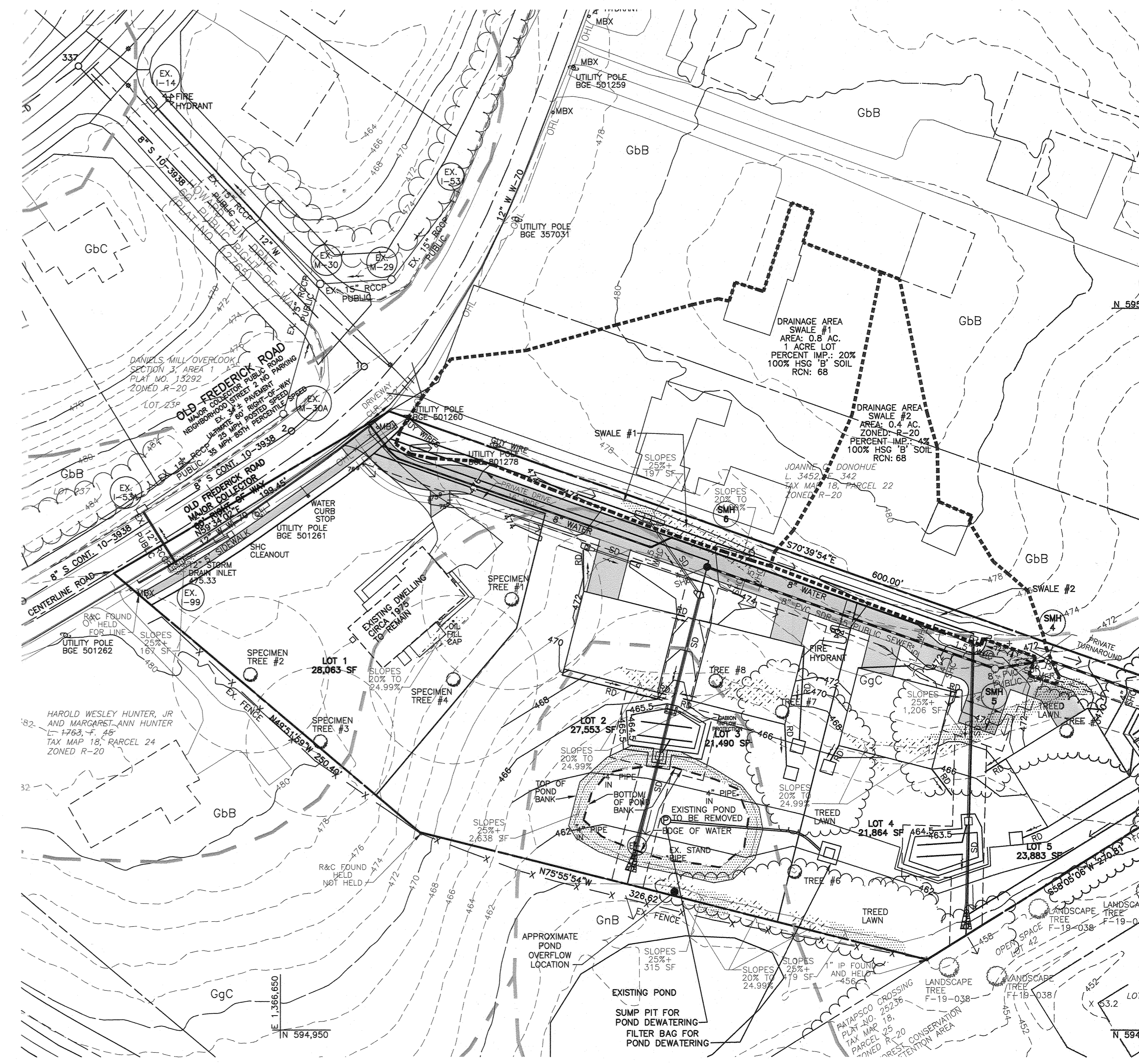
PERMANENT SWALES DRAINAGE AREA MAP
